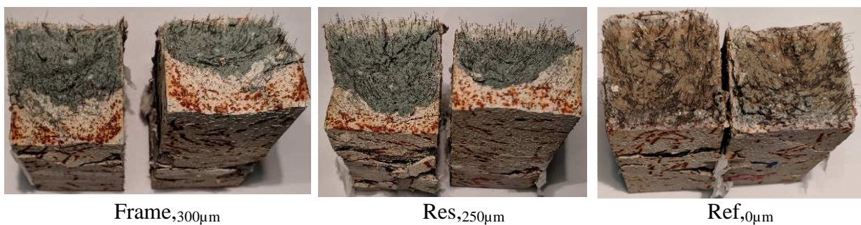
Figure 9: Corrosion of short steel fibres after wet-dry cycles.
