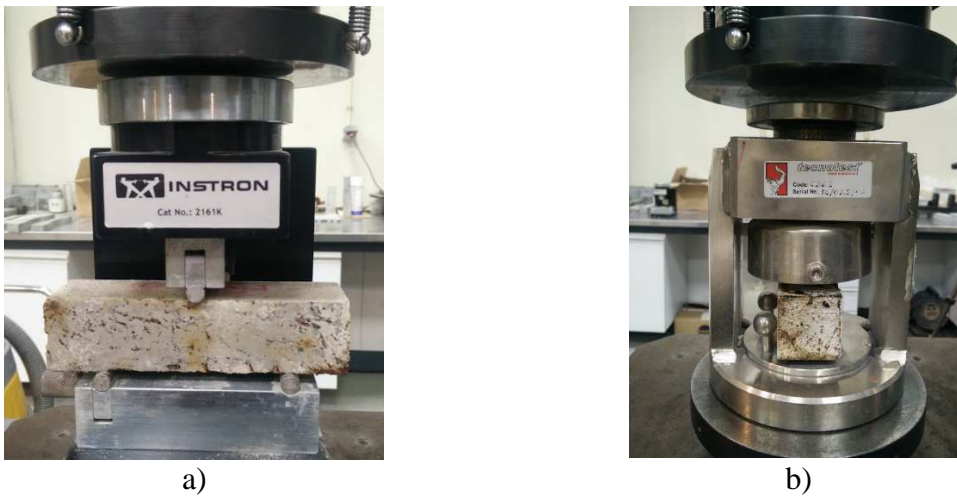
Figure 2: Determination of strength at 9, 36 and 180 days according to EN 196-1 [7]: a) flexure strength (3 point bending); b) compressive strength.
