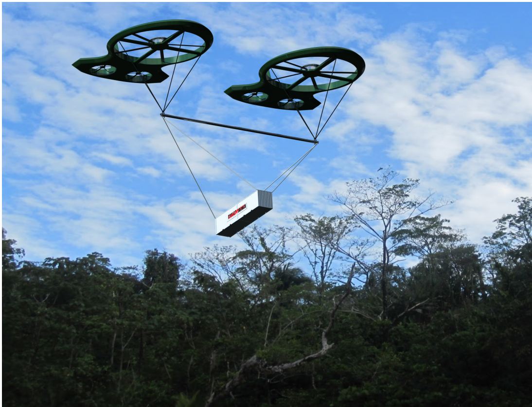
Figure 8.1: The Lift 2 system deploying a Hospitainer.
