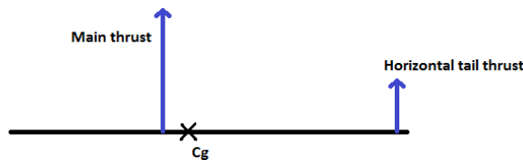
Figure 4.3: Longitudinal equilibrium around centre of gravity
