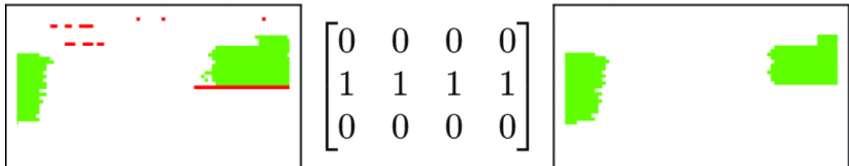
Figure 12: The box filter used to remove the outliers in potential dynamic points (Yoon et al., 2019).
