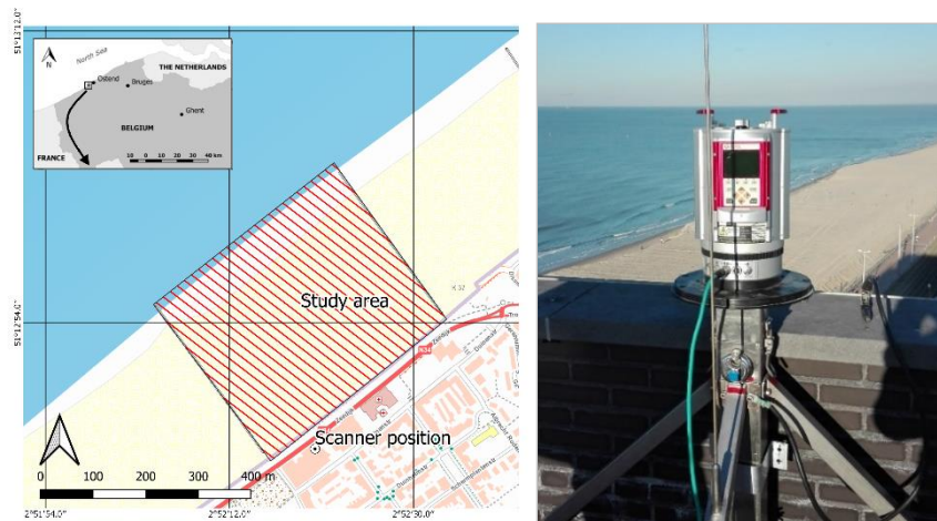
Figure 2. Map of the study area (left), Riegl® VZ-2000 TLS overlooking the beach (right)
