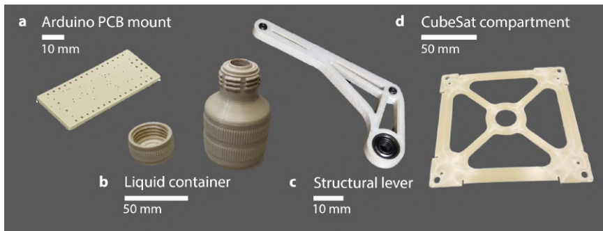
Figure 5.9 – Possible use cases of 3D-printed LCP in space, with different scales of application from left to right, manufactured with different 3D printers: A , an Arduino PCB mount, B , a screw-cap liquid container, C , a structural lever with bearings, and D , a compartment panel for a CubeSat.
