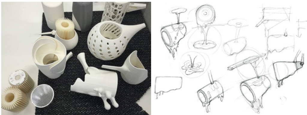
Figure 3 Early concept sketches trying to ‘break’ the mind-set of designing for injection moulding. Free-flowing organic shapes were promoted and prototypes were used to review with the company.
