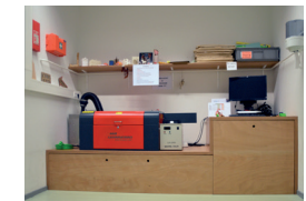
Laser cutters and others are equipped with a filter, like here at Apeldoorn. Caso.
