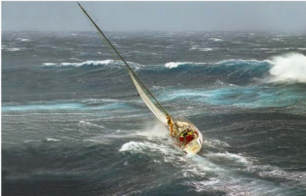
Figure 1.11: A sailing yacht in heavy weather with reduced sails to maintain a safe steady heel angle (Fretter, 2017)
