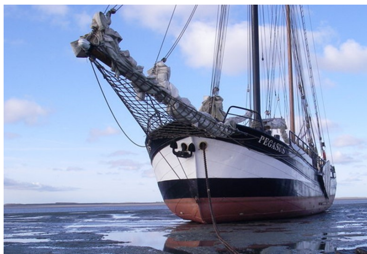
Figure 4.4: A typical Dutch sailing vessel with a shallow and square hullform with a wide beam (Windjammer Weltweit, n.d.)
