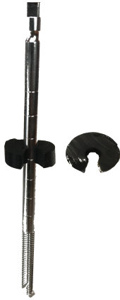
Figure 4.2: Depth utility prototype developed for LMICs, attached to fixator pin
