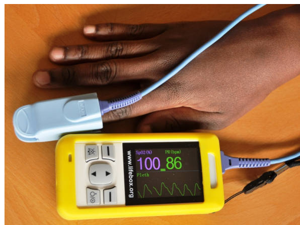
Figure 4.1: Pulse oximeter developed by Lifebox to enhance the safety of anaesthesia in LMICs
