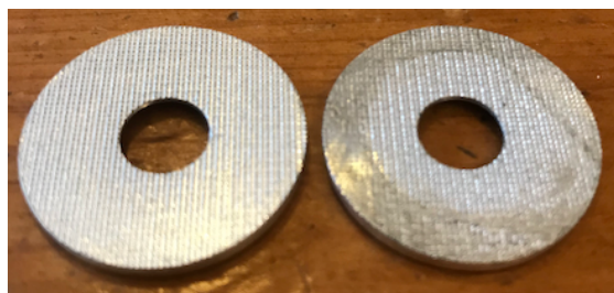
Figure 8. Plastic deformation of one of the friction disks of the universal clamp. Left: prior to testing, right: after testing.
