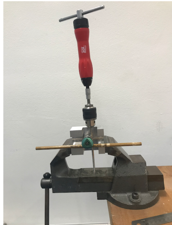
Figure 5. Hoffmann 3 clamp fixed in the test setup for fixator-pin and connecting-bar rotation.
