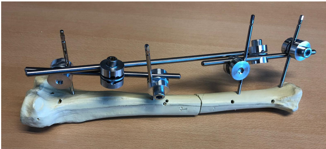
Figure 4.4: The three-way clamp prototype, the developed product in a first collaboration between the TU Delft and GSA.
