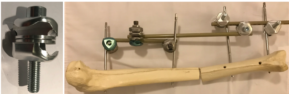
Figure 10.7: On the left, the universal clamp prototype. On the right a tibial open fracture model treated with a hybrid external fixation, consisting of three universal clamps and three Hoffmann 3 clamps.
