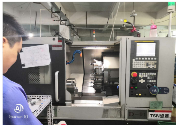
Figure 10.6: The five-axis CNC milling machine (Japan Fanuc) used by Tosony B.V. to manufacture four of the external fixator clamp prototypes.
