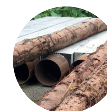
Wooden foundation piles Sustainable and low CO2 foundation
