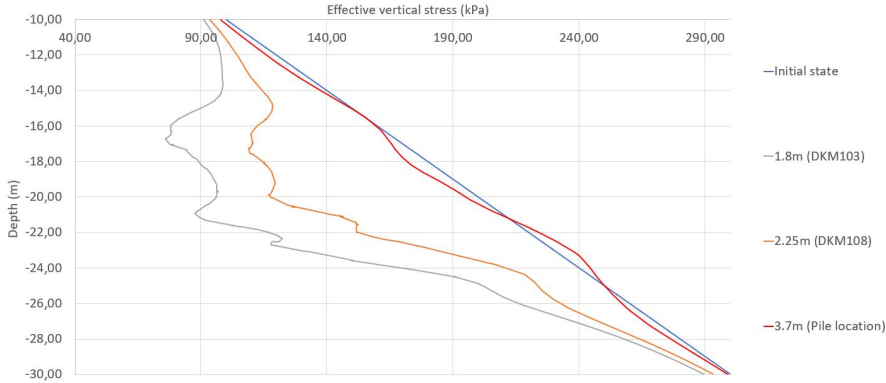
Figure 7.8: The vertical effective stress relief by 15 percent volume loss between -15m and -25m depth for the borehole in Lisse
