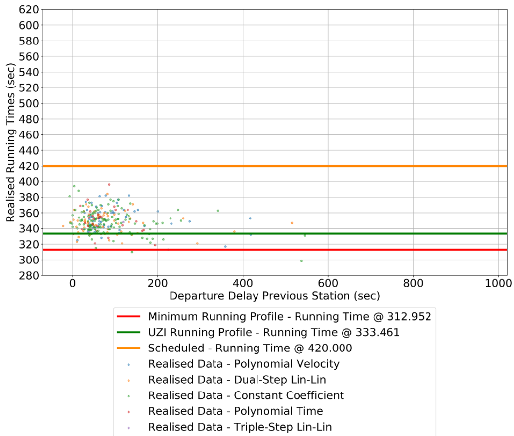
Figure L.5: Scatter Plot Comparative Analysis Departure Delay vs Realised Running Times - Brake Variant Highlight - Gdm
