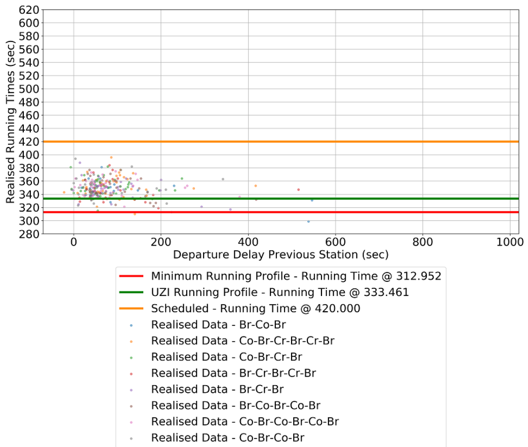
Figure L.6: Scatter Plot Comparative Analysis Departure Delay vs Realised Running Times - Deceleration Regime Highlight- Gdm
