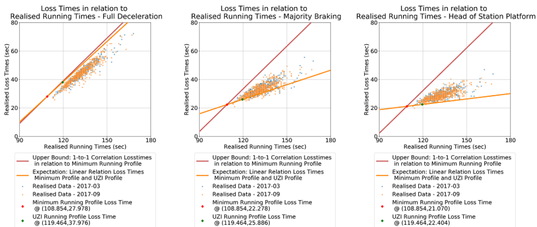
Figure L.36: Scatter Plot Comparative Analysis Realised Running Times vs Deceleration Loss Times - Seasonality High-light - Htn
