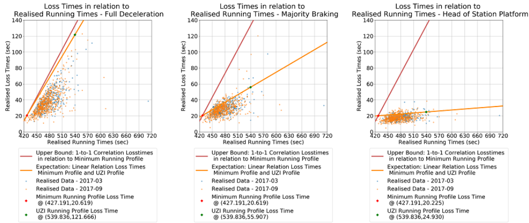
Figure L.40: Scatter Plot Comparative Analysis Realised Running Times vs Deceleration Loss Times - Seasonality Highlight - Zbm
