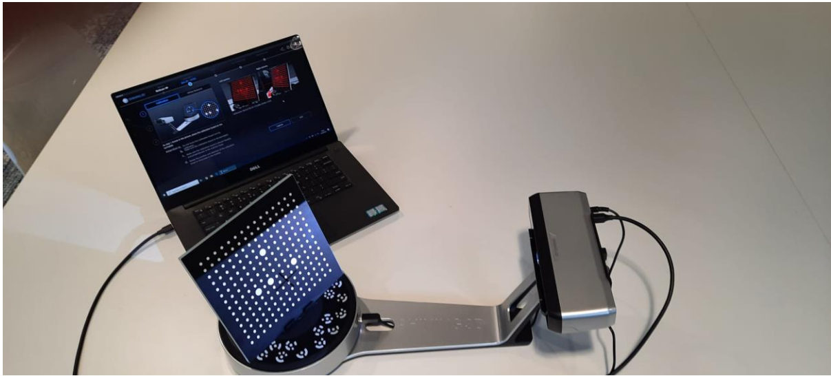
Figure 3: The EinScan SP V2 by Shining 3D, shown here during calibration. On the right is the camera used to create the 3D scan, currently attached to a turntable at a fixed distance. On the left the turntable with on it the calibration board used during the calibration process. The camera is attached to the laptop via USB-C for software processing purposes, such as calibration and (post)-processing of recorded 3D models.
