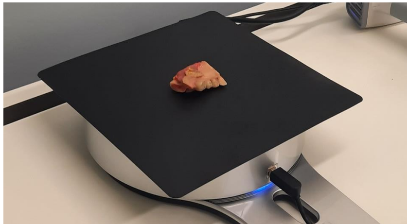
Figure 5: Cadaveric maxilla specimen on a sheet of matte black plastic ready for scanning. Here placed on top of the turntable of the EinScan SP.
