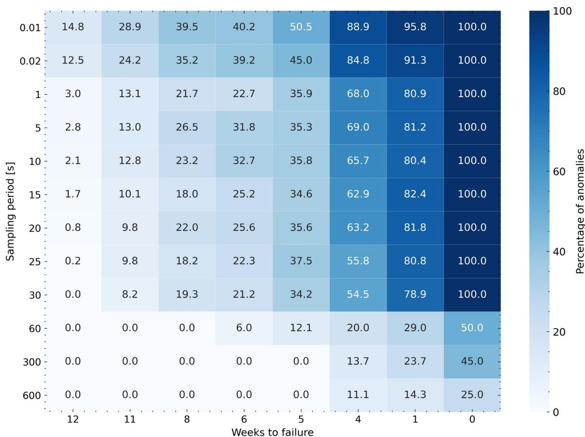
Figure 6.12: Heatmap for the percentage of anomalies detected by OC-SVM for different SCADA sampling rates for each week before failure
