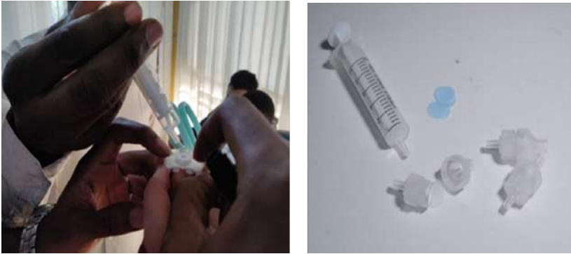
Figure 7.8: The difficulty of using the customized holder (Left) and the standard filter and filter holder (right)
