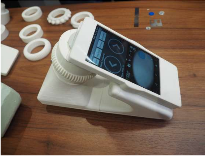
Figure 8.8: A second design of Excelscope 2.0 for imaging of parasitic diseases. System has the capacity to resolve 1 \mu\text{m} sized parasites. Device was developed as a master project at the faculty of industrial Design based on the concept proposed in (chapter 4 of this thesis)
