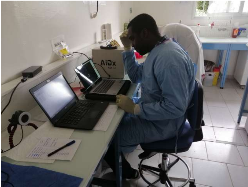
Figure 8.9: AiDx assist, a working prototype of a multimodal imaging device for malaria detection. The development of the functional prototype was co-ordinated by a non-profit Medical Optics fund, based on the concepts proposed in this thesis. The developed prototype was being tested for the quick diagnosis of Loa loa and malaria parasite in prepared blood samples at the CERMEL (Center of Medical Research Lambaréné) laboratory facility in Lambarene, Gabon. Picture was taken in January 2020.
