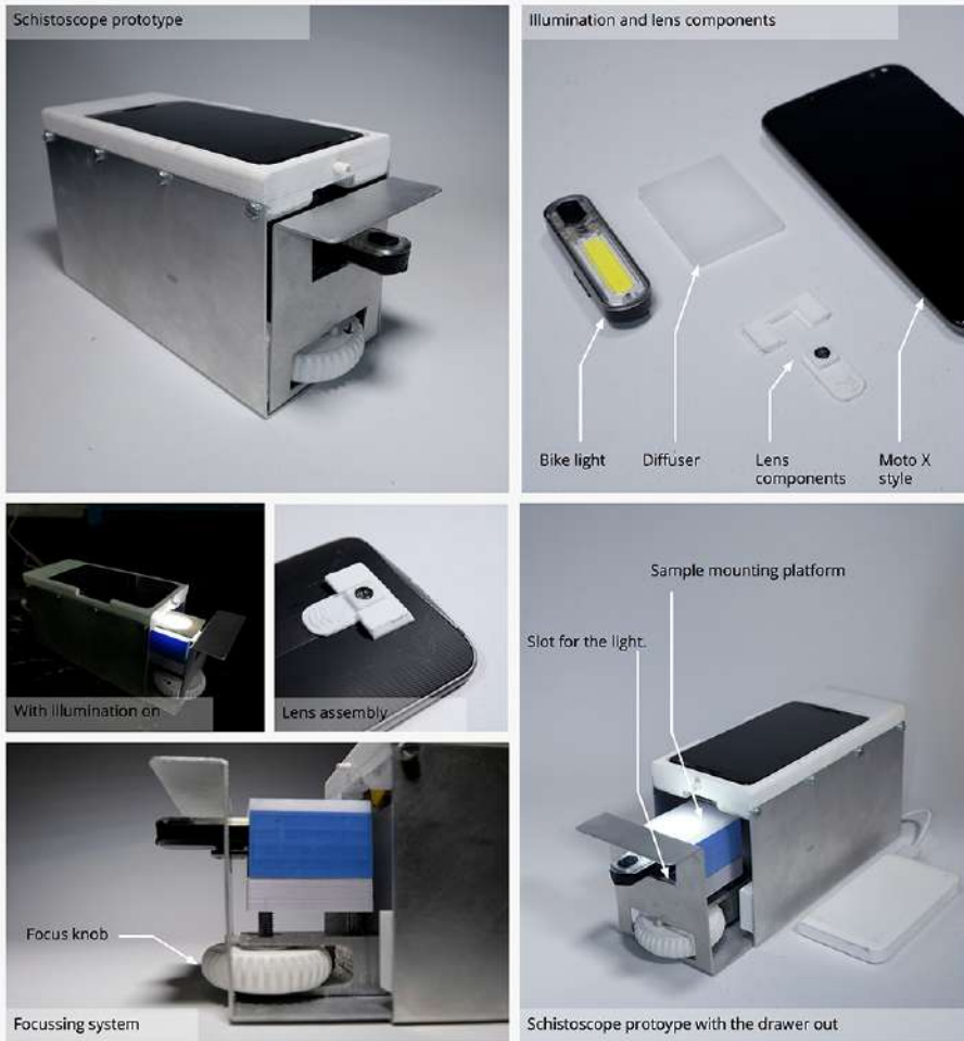
Figure 4.12: Assembly parts of the final iteration of the device. Parts are fabricated using 3D printed parts, locally sourced components and low-cost aluminium sheet.
