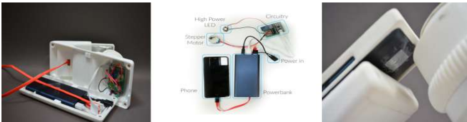
Figure 5.9: Overview of the system design (a) depicts the battery back up and micro-controller used for the digital control of the stepper motor (b) shows the circuitry while (c) depicts the attachment of the ball lens mounted in a piece of aluminum foil and attached to the smartphone with a scotch tape.
