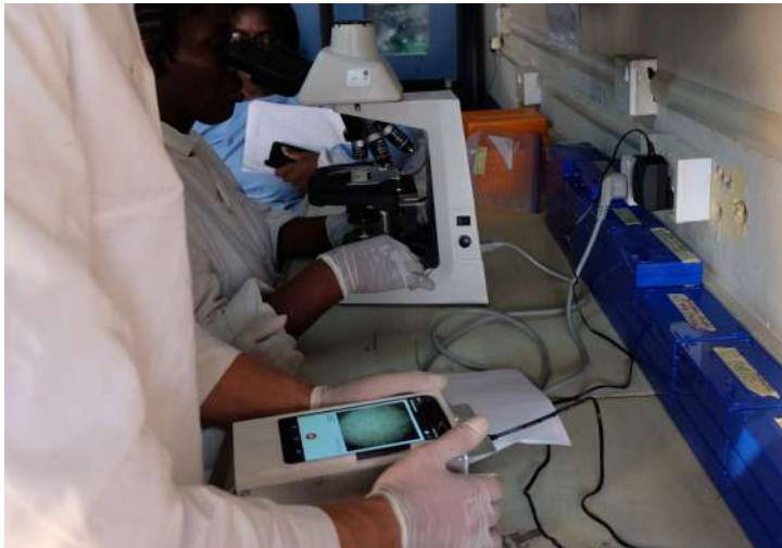
Figure 8.4: Working prototypes used to image Schistosoma haemtobium at the ANDI Malaria research centre in Lagos, Nigeria. An expert is seen looking through a standard microscope while the developed cellphone based microscope also provides automated detection of the eggs (2018).
