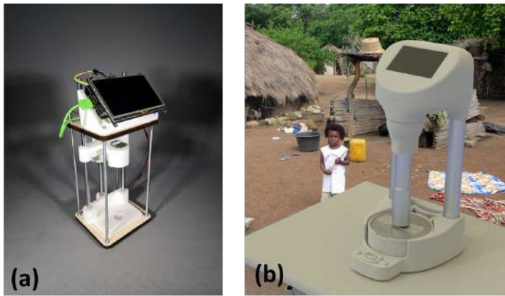
Figure 8.3: Developed automated microscope using low-cost consumer grades electronics and optics based on the methods described in Chapter 3. It is a simplification of the WHO approved diagnostic method and requires minimal technical skill, we envisage that this methodology will be of practical interest to the primary health care community. (a) shows the first working design of the prototype and (b) is the designed implementation. Functional Prototype was developed as a master project at the faculty of industrial Design based on the concept proposed in (chapter 4 of this thesis).
