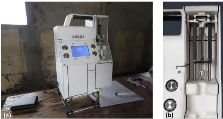
Figure 3.17: (a) Is the complete diagnostic device and (b) shows the sample injection chamber where the syringe containing 12 ml of infected urine sample is mounted. The urine is pumped through the micro-channel flow-cell by an attached stepper motor to provide accurate and consistent flow. 1.3 ml of the sample is used to flush out particles from the micro-channel flow cell.
