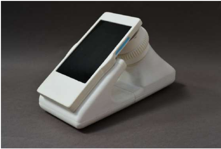
Figure 5.8: Motorized prototype with automated x-y movement of blood sample, which enables fast acquisition of large number of images.
