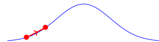
Figure 3.1: A Markov chain walks along the landscape of a probability distribution. It compares the current height of the distribution to the height of a possible new position. If the new position is located higher up the hill it is more likely to accept the new position, otherwise it stays in place.
