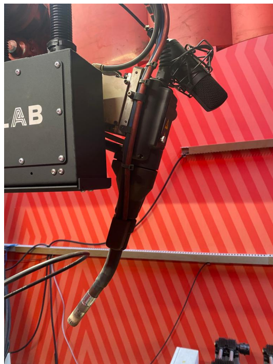
Figure 1. Attachment of microphone to welding arm.
