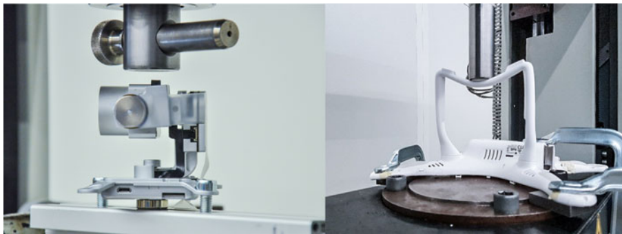
Figure A1. Static compressive test to determine the force–deformation curve of each component.
