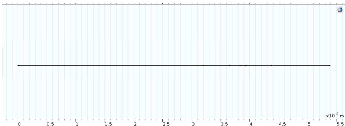
Figure 2.6: 1D layer geometry of a PV module built and simulated in COMSOL. From left to right, the layers between the nodes are glass, EVA, c-Si, aluminium, EVA, Tedlar.
