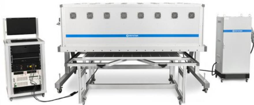
Figure 4.1: Large Area Solar Simulator used to determine the influence of the PCM on the PV module temperature. Photograph extracted from [49].
