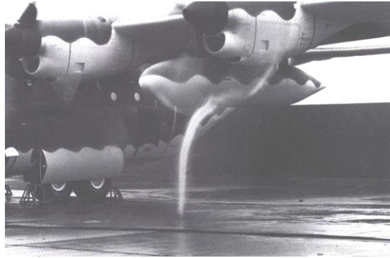
Fig. 1 Occurrence of ground vortex on the outboard propeller of aircraft C130 [13] (This figure is taken from NASA SP-514 [J. F., Campbell, and J. R., Patterns in the sky-natural visualization of aircraft flow fields] and used with permission of NASA).
