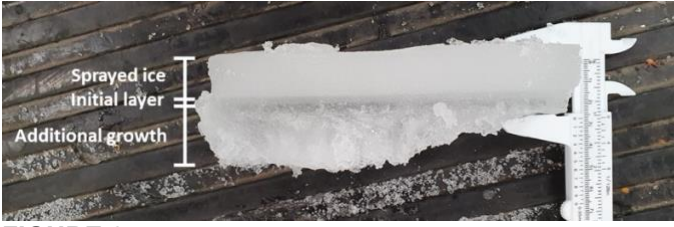
FIGURE 6: ICE VERTICAL CROSS SECTION AT THE END OF A TEST DAY (17-6-2021): A SPRAYED LAYER ON TOP, A LAYER OF INITIAL ICE THAT WAS FORMED BEFORE THE START OF THE SPRAYING PROCESS IN THE MIDDLE, AND A LAYER OF ADDITIONAL ICE GROWTH AT THE BOTTOM.
