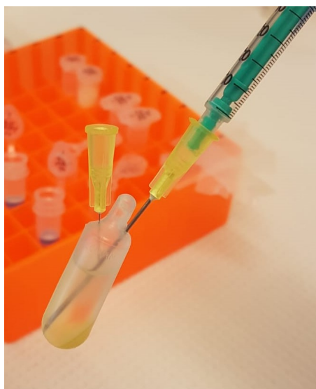
Figure 3.2: Needles in ultracentrifuge tube to remove supernatant with a syringe. The second needle is placed to prevent the occurrence of a vacuum.
