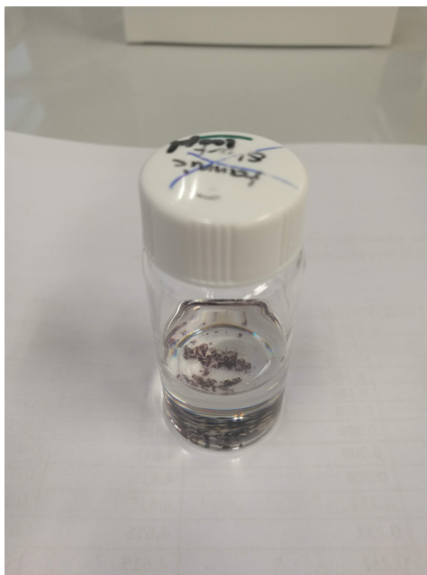
Figure B.5: Not well mixed LSC sample. When the counting vial is not immediately swerved after addition of the sample to the counting cocktail, the sample sticks to the bottom of the counting vial. It is not possible to dissolve this later in time.
