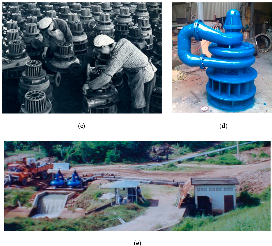
Figure 5. Different types of water turbine-pumps (WTPs): (a) Hydraulic converters installed in the Muffatwehr at the Isar River in Munich [81]. Reproduced with permission from Springer Nature. © Springer Nature ( https://doi.org/10.1007/978-3-642-50802-8_18 ); (b) Schematic view of the typical installation of a WTP [14]. Reproduced with permission from Food and Agriculture Organization of the United Nations © FAO ( http://www.fao.org/3/ah810e/AH810E12.htm#12.1 ). A from the original; (c) Mass production of Chinese water turbine-pump (CWTP). Reproduced with permission from Gejing Jiang. © 有金华天阳电子有限公司 ( http://www.jiaxiangwang.com/cn/guizhou.htm ); (d) Multi-stage Vietnamese hydraulic pump [116]. © Viện Khoa học Thủy lợi Việt Nam ( http://www.vawr.org.vn/index.aspx?aac=CLICK&aid=ARTICLE_DETAIL&ari=2314&lang=1&menu=&mid=-138&pid=1&title=cong-nghe-bom-thuy-luan-bom-nuoc-tu-dong-phuc-vu-nong-nghiep-mien-nui-va-trung-du ); (e) Globe case coaxial water turbine pumps commissioned in the Mae Phum Reservoir, Phayao province, Thailand [117]. © Royal Irrigation Department. CC BY-NC-SA 3.0. Cropped from the original.
