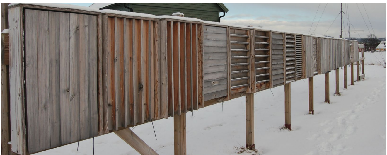
Fig. 23. Photo showing the south facing structural frame at Voll, Trondheim used for Hirche's experimental research. From Wood Weathering as Design Option (Hirche, p. 76), by M. Hirche, 2014, Norwegian University of Science and Technology. Copyright [2014 by Majbrid Hirche.
