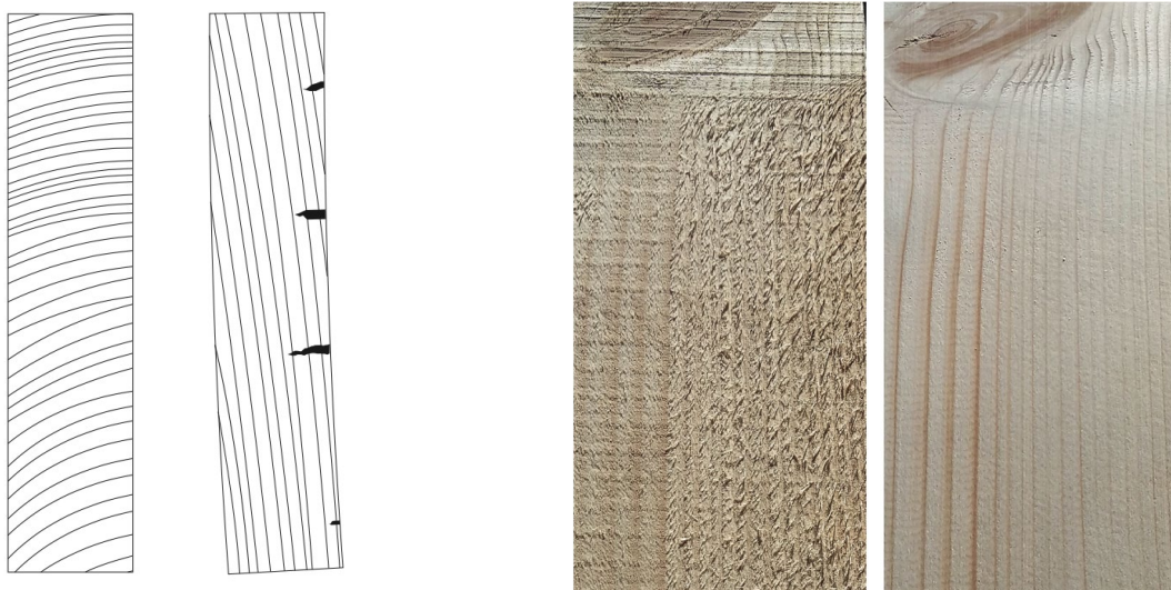
Fig. 7. (left) Vertical grain cladding boards will have greater dimensional stability and be less likely to develop cracks than flat-grain cladding boards. From Weathering of unpainted wooden façades - Experience and examples (Zimmer et al., p. 15), by Norwegian University of Science and Technology, 2014.
