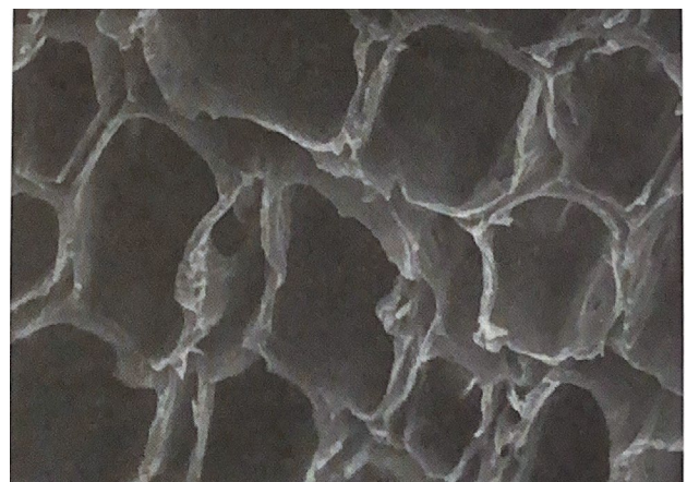
Fig. 12. (left) Southern pine cross-section (1000x). (right) Southern pine cross-section following 1000h of UV radiation ( \lambda > 220 nm, 1000x). From "Handbook of Wood Chemistry and Wood Composites" , by CRC Press, 2005.
