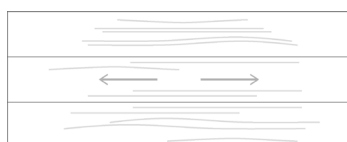
WATER MOVEMENT ALONG THE FIBRES
