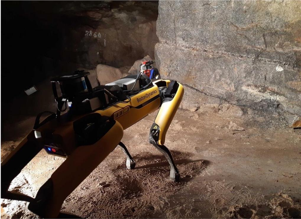
**Figure 3.6.** Underground application setup in Floz 8 at Zinnwald/Cinnovec mine with Spot and payload instruments facing UG-1 rock surface.
