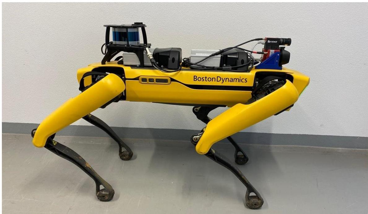
**Figure 2.3.** Side view of Spot with two CORE computers, Cubert X20P hyperspectral camera and VLP16 LiDAR fully mounted.
