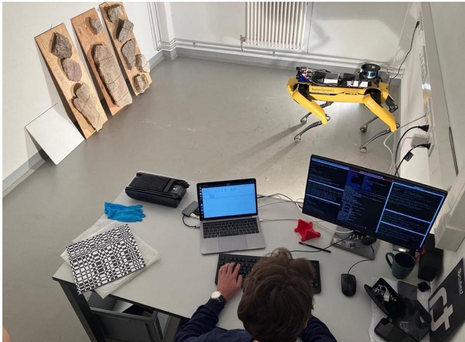
**Figure 3.3.** Lab test setup showing the rock samples on three wooden boards, Spot, and light setup behind Spot on either side.
