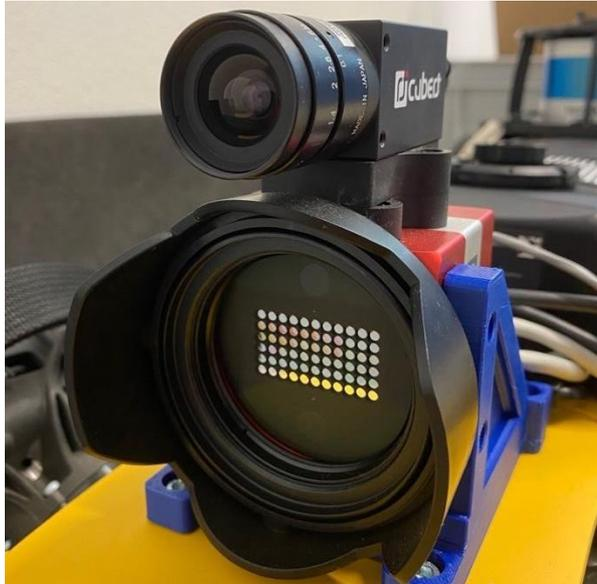
**Figure 2.4.** Cubert X20P spectral camera suboptic lens (below) and panchromatic lens (top).
