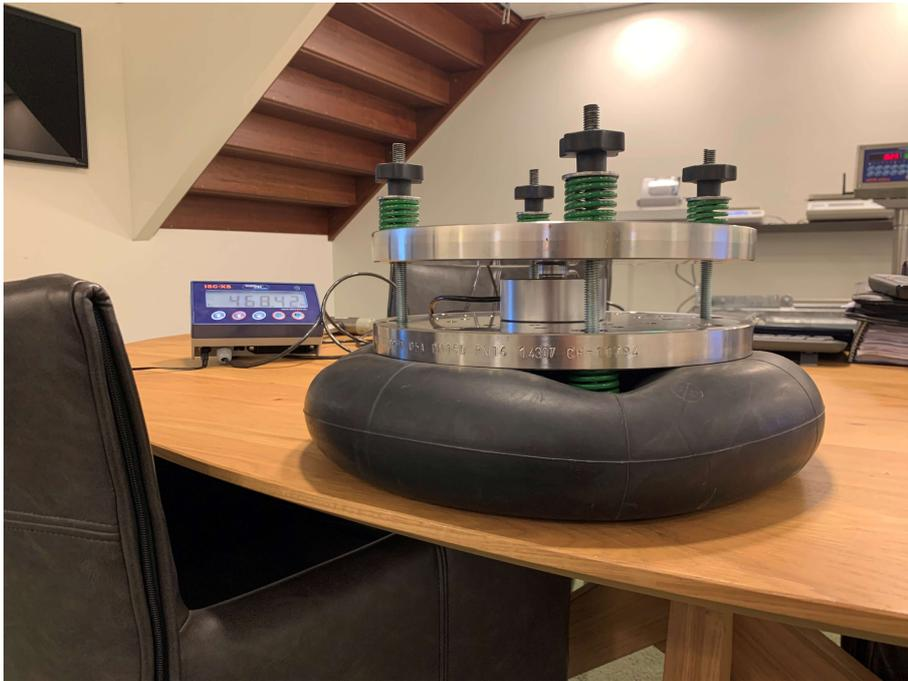
Figure D.2: Measurement of the spring force at Henk Maas Weegschalen B.V.
