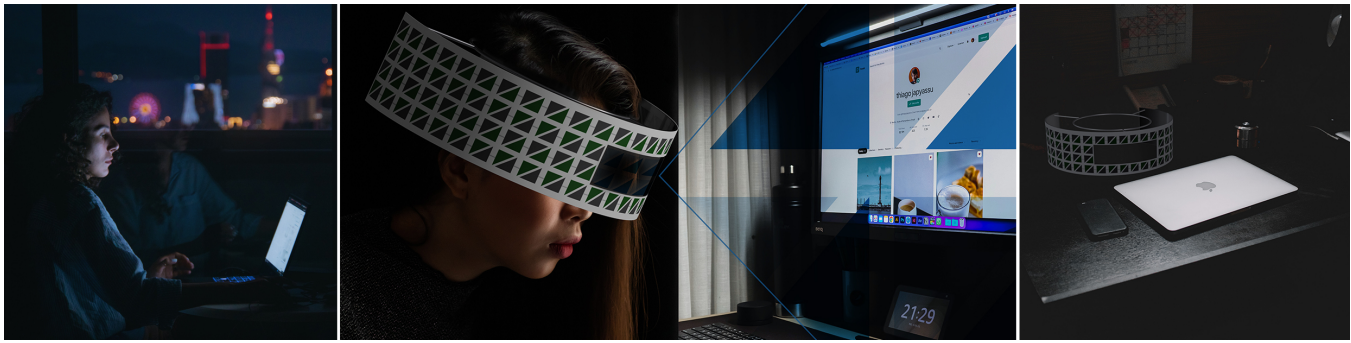
Figure 15: Circadian Navigator : As the cyano unit of the artefact reacts to the light emitted from the screen, the EC component would darken its colour which would subsequently restrict the opacity of the worn lenses (i.e., visibility), nudging the wearer away from their screen use.
