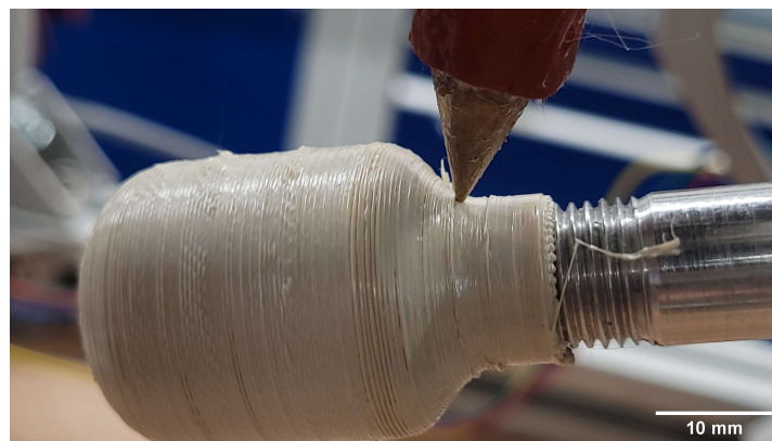
Figure 5.25: An ironing pass is executed, where the nozzle follows the outer contour of the part without extruding. Small chips of overextrusion are removed.
