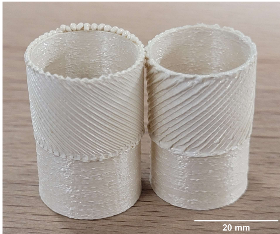
Figure 5.11: Cylinder with -45 (left) and 45 (right) degrees overwrap, the bottom section of the cylinder cannot be reached by the nozzle when printing normal to the cylinder
