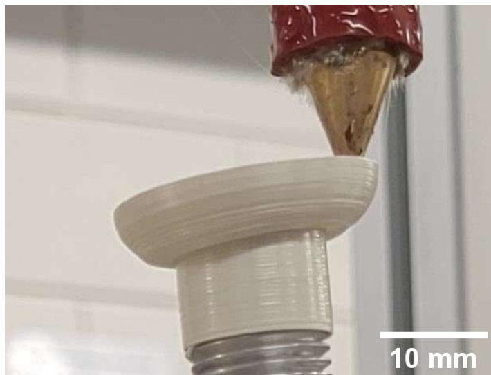
Figure 5.22: In some instances the liner detaches from the base cylinder during printing, when the liner is printed before the fillet.
