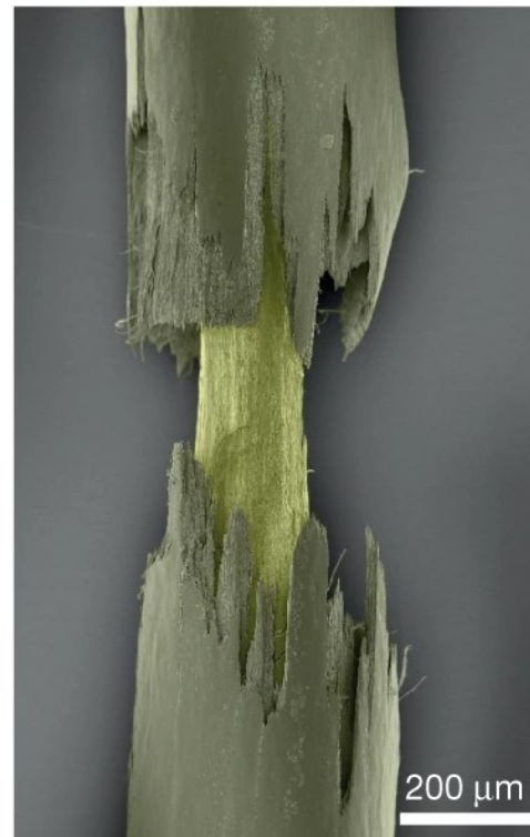
Figure 2.2: An electron microscopy image of a printed filament presenting the core and shell structure [3]
