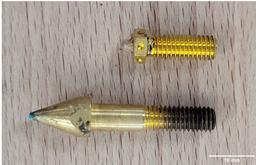
Figure 5.6: Comparison of short and long nozzle, top is standard E3D Volcano V6 0.4mm nozzle, bottom is extended 0.4mm nozzle [43].
