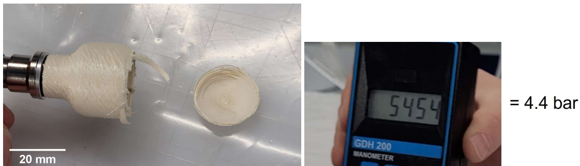
(a) Failure of the first specimen
