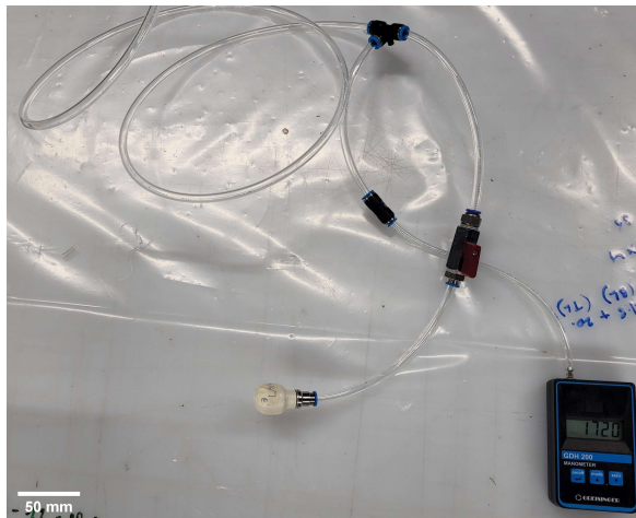
(a) The pressure lines connected to the pressure vessel, the pressure line in the top left feeds to the pressure regulator, figure b, a valve is placed just in front of the pressure vessel. A digital pressure sensor is connected to the system.
