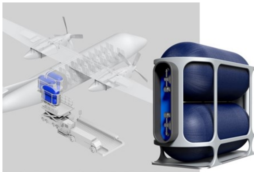
Figure 1.2: Cylindrical COPV mounted in a rectangular frame loaded in a passenger aircraft [2]
