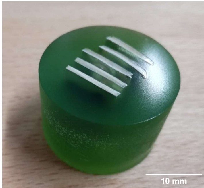
Figure 4.3: LCP samples have been potted in epoxy and polished for microscopy observation.
