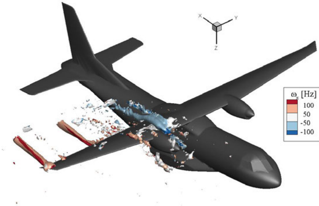
Fig. 7. Illustration of the vortical structures in the flow field. Iso-surfaces of Q-criterion ( Q = 1000 \text{ s}^{-2} ) color-coded by streamwise vorticity.
