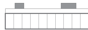
Figure 21 Single-loaded slab: Accommodation units positioned on single side with a corridor that connects to 2 shafts at both ends of the plan.
