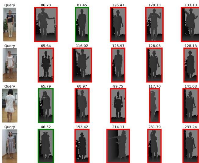
Figure 49: RobotPKU, One-stream network: Examples for query images (RGB) and corresponding gallery images (depth) with lowest distance.
