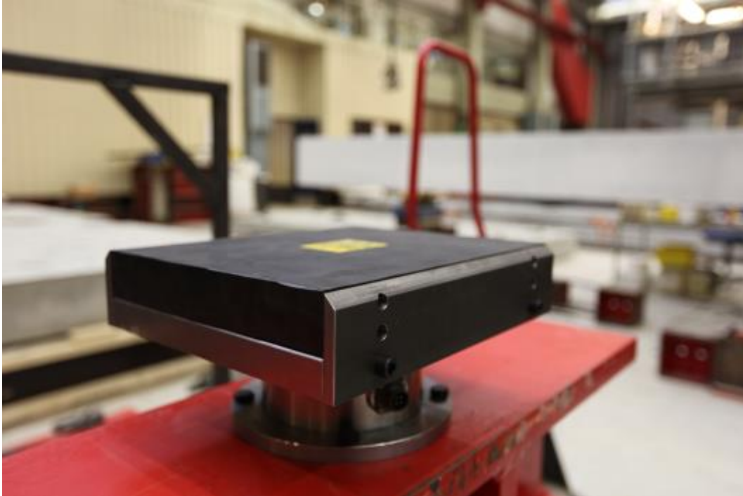
Figure 2. Example of elastomeric bridge bearings in laboratory conditions
