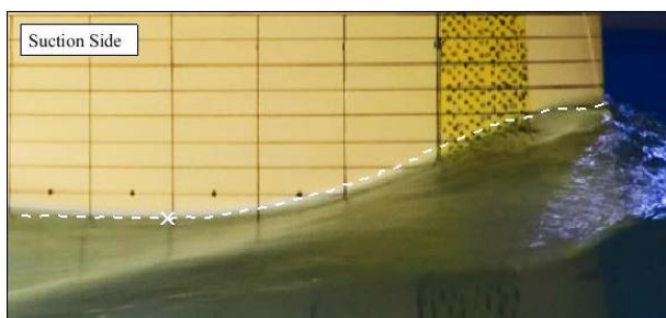
Figure 5 Bow wave profile corresponding to the median error ( Fn = 0.17 and \beta = 6^\circ ). The images have been overlaid with the wave elevation obtained by simulation.
