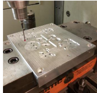
b) CNC milling of the moulds
