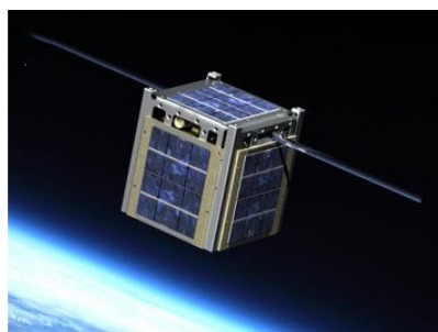
(b) Body mounted type where the solar cells are mounted on the satellite body
