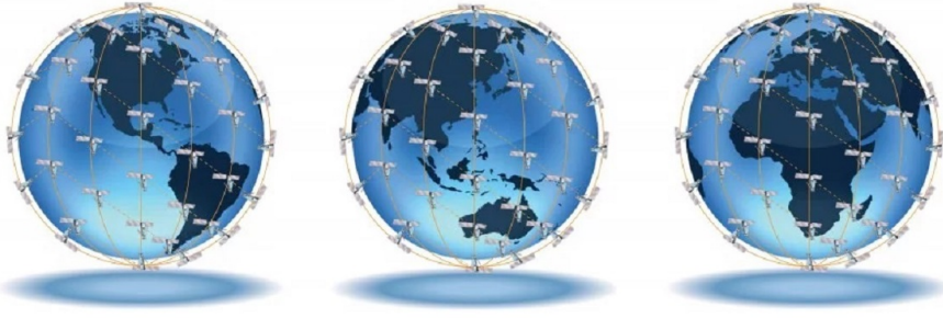
Figure 1.2: A glimpse of arrangement of satellites in the second generation Iridium NEXT constellation [6]
