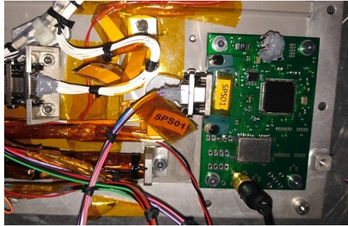
Figure 4.10: Placement of the \mu GPS receiver in the nanosatellite
