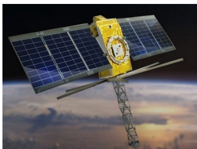
(a) Deployable type where the solar panels are deployed after launch
