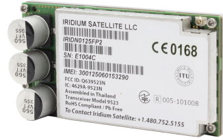
(b) Iridium 9523 module, a voice and data-based satellite transceiver module
