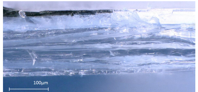
Fig. 8. Cross-section of actuator with 3 layers of spin coated polymer.
