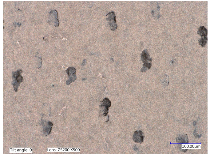
Fig. 4. 5 layers of sintered JS-B25P silver ink printed on Novele
