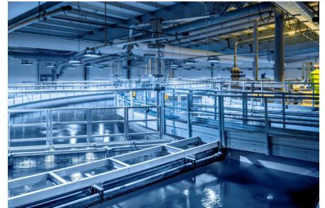
Figure 17 Nordic Aquafarm, located in Norway, uses RAS or recirculation tanks, a technology for farming fish by reusing the water in the production
