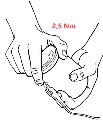
Figure 15 - maximum static torque with 2 hands p5 user ▲
