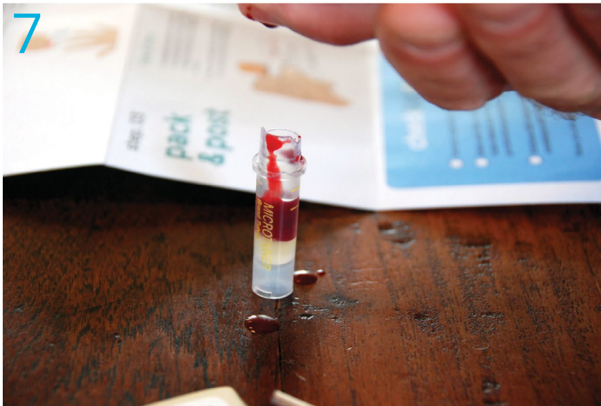
7 The user spills blood drops due to the container small inlet and instability of the hand.
