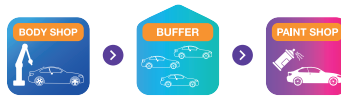
Figure 5.2: The structure of the simplified model: a body shop and a paint shop that share a buffer.
