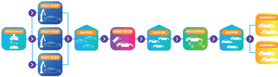
Figure 5.1: An example of an automotive productive line with five steps: a press shop, three parallel body shops, a paint shop, mounting and two separate assemblies. There are buffers between the body, paint, mounting, and assembly steps.
