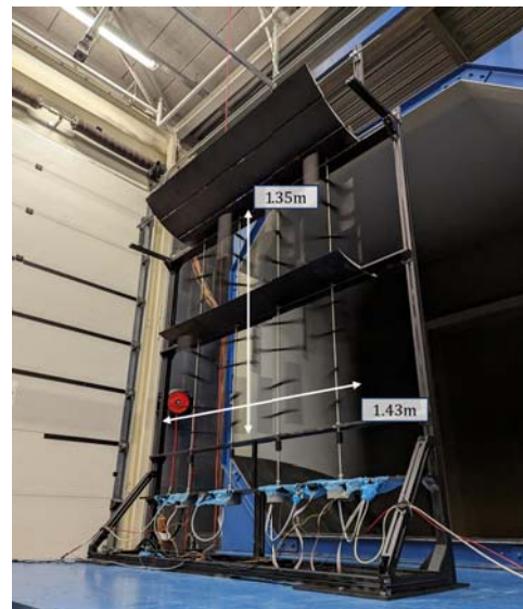
Figure 2. 3D Visualization of the Multi-Rotor System (MRS) with lift-generating wings. Full details in [Broertjes et al., 2024]
