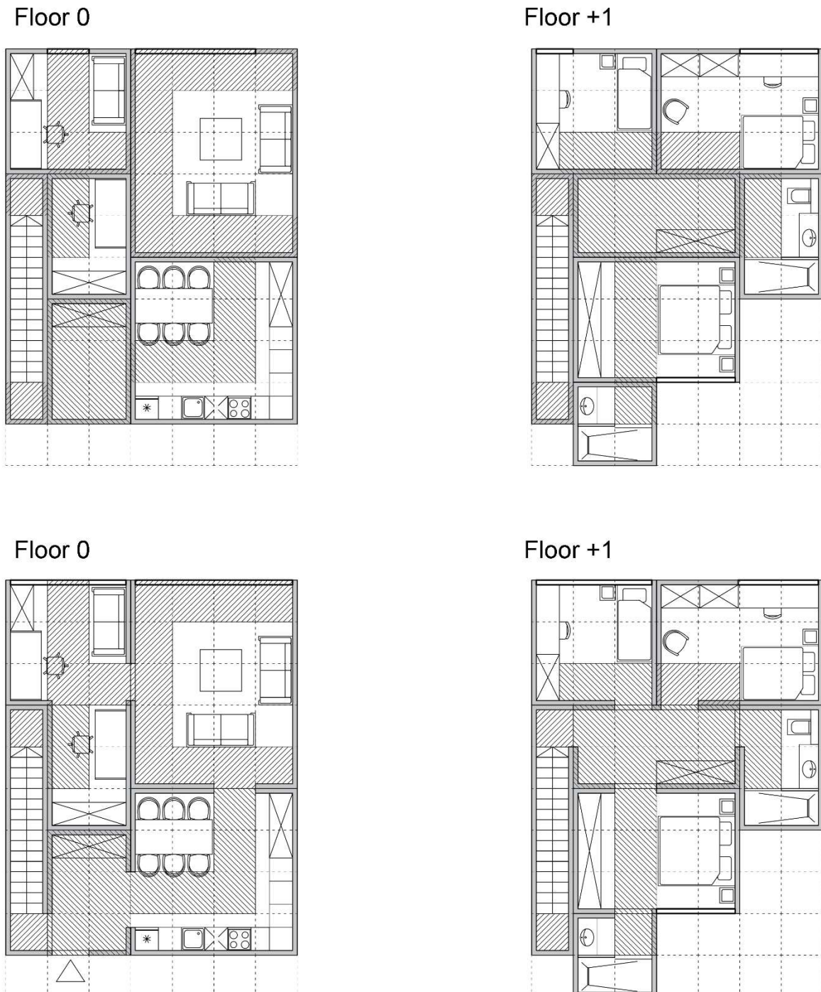
Fig. 23 Possible apartment configuration 1. Modules configured by the user on top. Apartment after placing openings below. Grid horizontal size 108 x 108 cm.
