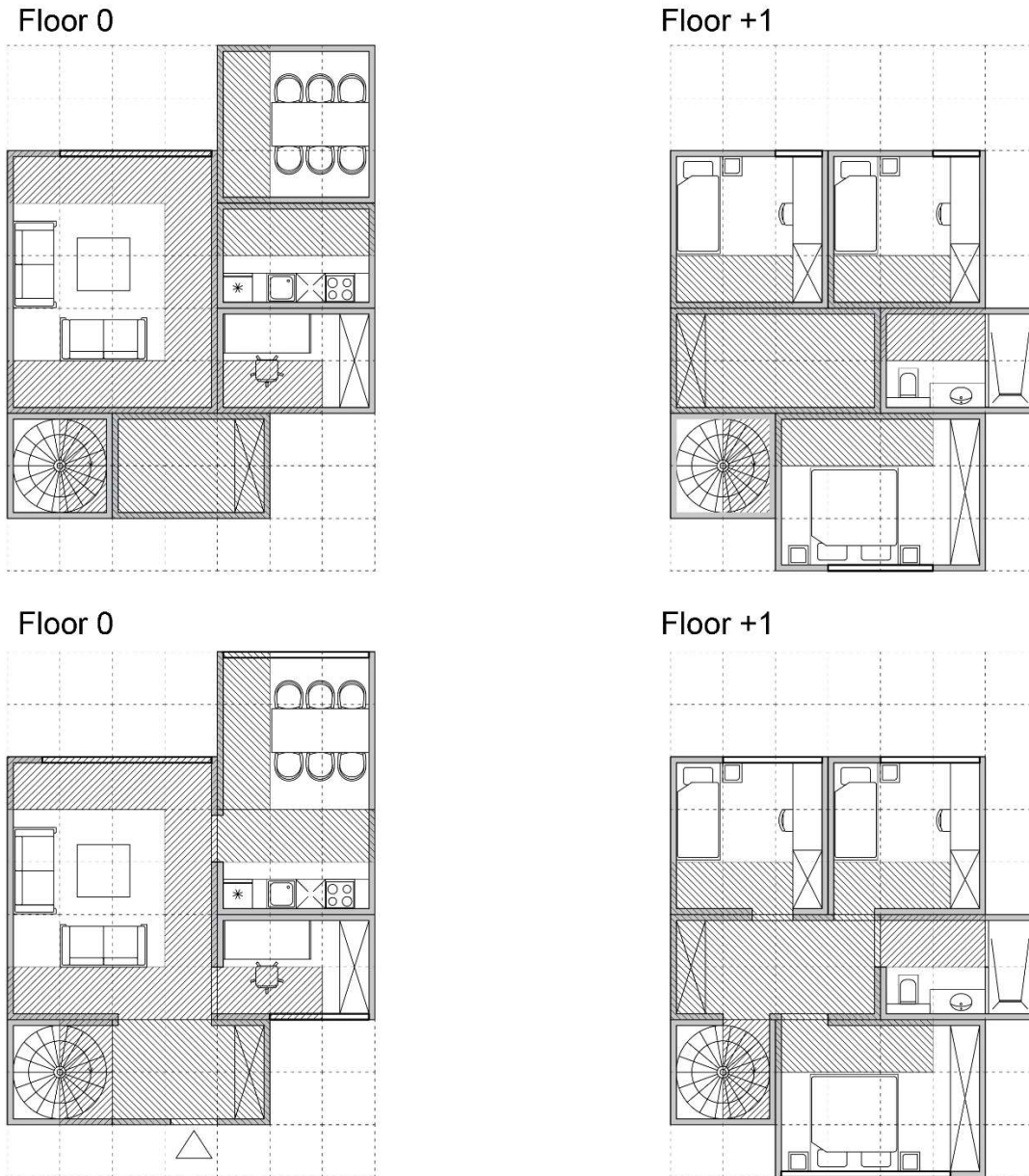
Fig. 24 Possible apartment configuration 2. Modules configured by the user on top. Apartment after placing openings below. Grid horizontal size 108 x 108 cm.
