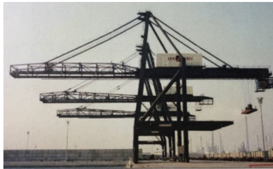
Figure 2.2: Modified A-frame dockside crane from Sea-Land [12]
