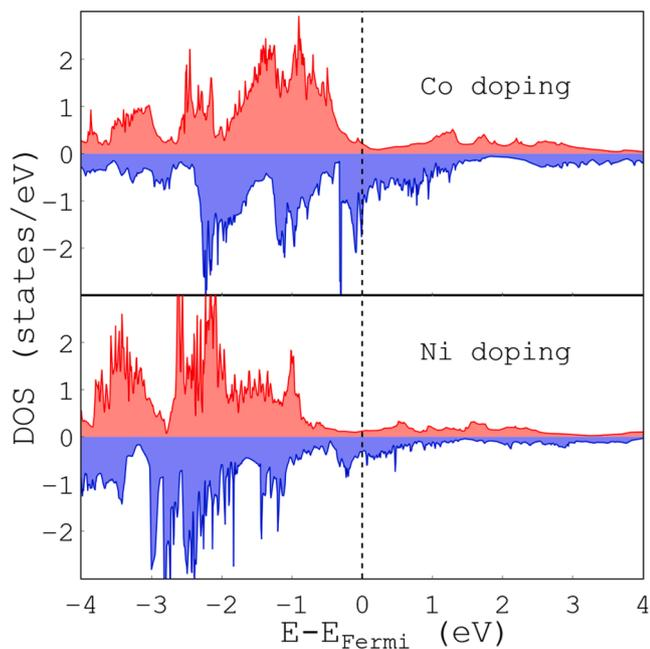
Fig. 11. Partial DOS of  $Mn_{0.66}Fe_{1.25}T_{0.08}P_{0.66}Si_{0.33}$  ( $T = Co, Ni$ ) compounds for Co and Ni in the vicinity of Fermi level. Spin up and spin down states are coloured with red and blue respectively. Zero represents the Fermi energy.
