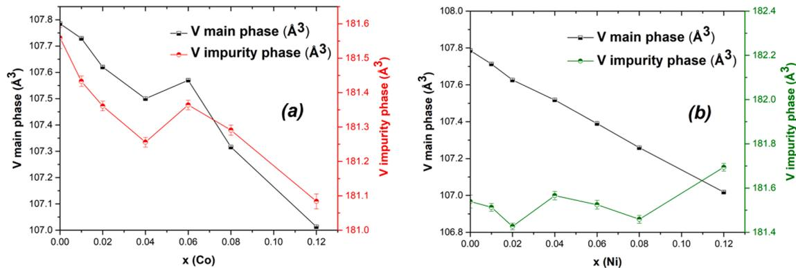
**Fig. 4.** Composition dependence of the volume (main phase and impurity phase) of the (a) Mn<sub>0.62-x</sub>Fe<sub>1.33</sub>Co<sub>x</sub>P<sub>0.66</sub>Si<sub>0.34</sub> and (b) Mn<sub>0.62-x</sub>Fe<sub>1.33</sub>Ni<sub>x</sub>P<sub>0.66</sub>Si<sub>0.34</sub> derived from X-ray diffraction patterns measured at 348 K (PM state).
