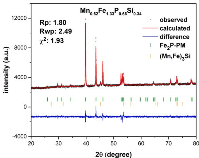
Fig. 3. Observed and calculated XRD patterns of  $\text{Mn}_{0.62}\text{Fe}_{1.33}\text{P}_{0.66}\text{Si}_{0.34}$ .
