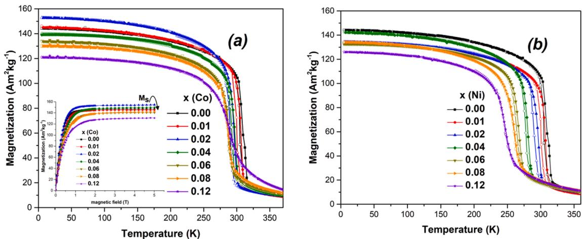
Fig. 7. Temperature dependence of the magnetization of (a)  $\text{Mn}_{0.62-x}\text{Fe}_{1.33}\text{Co}_x\text{P}_{0.66}\text{Si}_{0.34}$  and (b)  $\text{Mn}_{0.62-x}\text{Fe}_{1.33}\text{Ni}_x\text{P}_{0.66}\text{Si}_{0.34}$  compounds measured in a magnetic field of 1 T. The insert shows the field dependence of  $\text{Mn}_{0.62-x}\text{Fe}_{1.33}\text{Co}_x\text{P}_{0.66}\text{Si}_{0.34}$  measured at 5 K.
