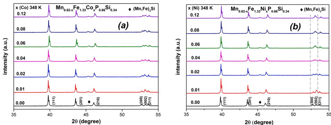
**Fig. 6.** X-ray diffraction patterns of (a) Mn<sub>0.62-x</sub>Fe<sub>1.33</sub>Co<sub>x</sub>P<sub>0.66</sub>Si<sub>0.34</sub> and (b) Mn<sub>0.62-x</sub>Fe<sub>1.33</sub>Ni<sub>x</sub>P<sub>0.66</sub>Si<sub>0.34</sub> recorded at 348 K (PM state). With increasing Ni content, the (300) and (002) reflections shift towards each other, indicating that the lattice parameters  $a$  and  $c$  move in opposite direction.
