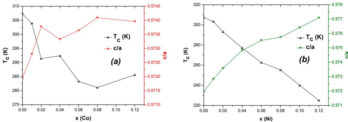
**Fig. 5.** Composition dependence of the  $T_c$  upon heating and  $c/a$  ratio derived from X-ray diffraction patterns measured at 348 K (PM state) of the (a) Mn<sub>0.62-x</sub>Fe<sub>1.33</sub>Co<sub>x</sub>P<sub>0.66</sub>Si<sub>0.34</sub> and (b) Mn<sub>0.62-x</sub>Fe<sub>1.33</sub>Ni<sub>x</sub>P<sub>0.66</sub>Si<sub>0.34</sub>.
