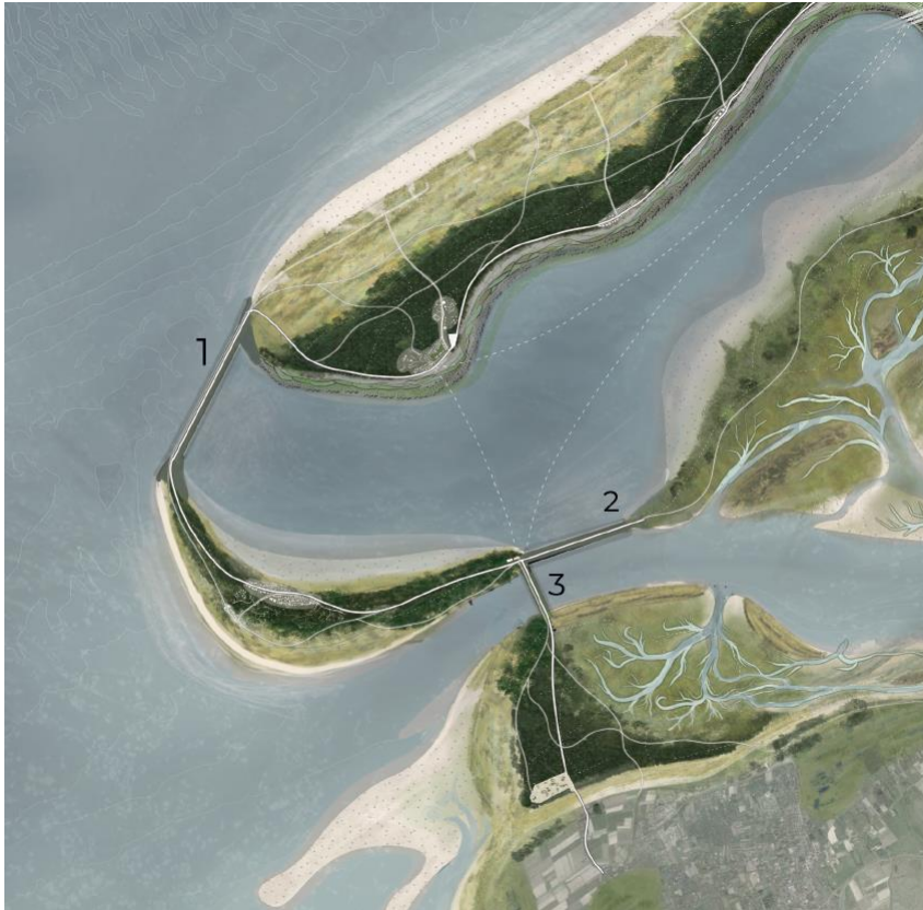
Figure 8: Zoomed in view of the hydraulic structures as part of the Delta21 plan, 1 is the energy storage lake outlet to the north sea, 2 is the spillway to the energy storage lake, and three is the new storm surge barrier.
