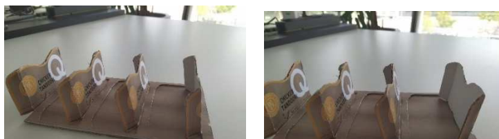
Figure 180: At the beginning of the test (left) the front baffle returned to its original position. At the end of the test the front baffle did not fully return to its original position anymore. (right)
