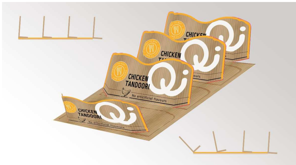
Figure 8: The baffles can bend forward to make sure a smooth placing and picking motion is possible.
