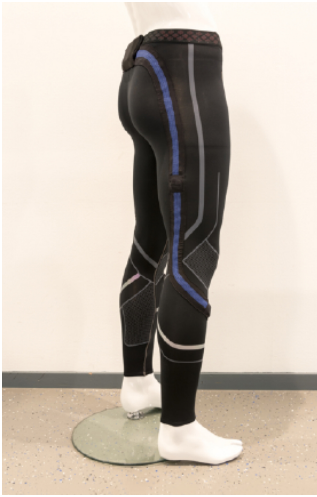
Figure 1.2: Sensor trousers prototype with fully embedded sensors developed within subproject P1 of the CAS program. Taken from [1].
