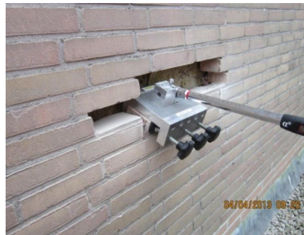
Figure 23: Lever Test Determination of Bond Strength @nebest
