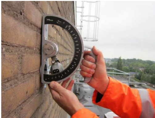
Figure 19: Determination of Joint Hardness Using Pendulum Hammer @nebest
