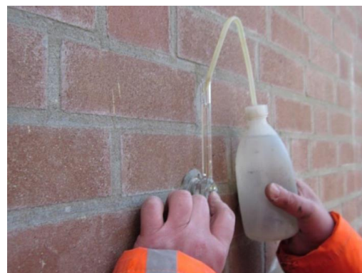
Figure 21: Testing Tube of Karsten @nebest
