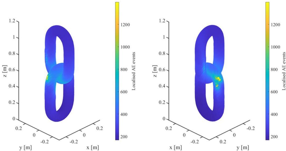
**Fig. 7.** Localisation map of AE sources calculated for a testing period of 5 hours.
