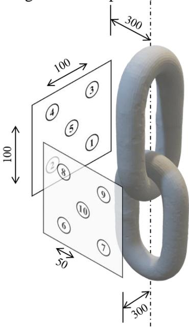
**Fig. 3.** Schematic illustration of the layout of the AE transducers. Group 1 includes sensors 1-5. Group 2 includes sensors 6-10. Dimensions in mm.
