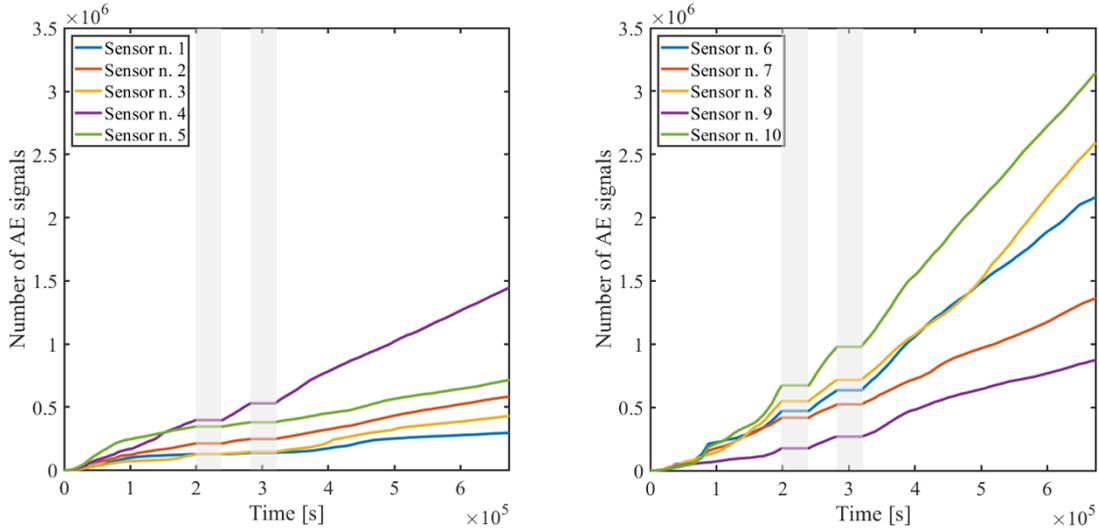
**Fig. 5.** Cumulative number of AE signals measured by each sensor. Grey areas indicate the periods where measurements are not available.
