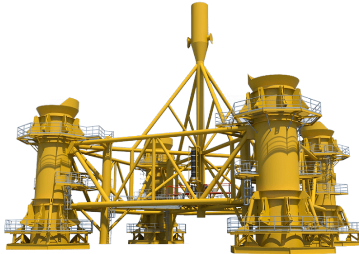
Figure 2.1: Alternative pre-piling template design
