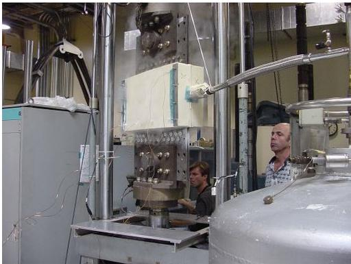
(a) Sequential bi-axial testing under cryogenic conditions presented in the study of Robinson et al. [86]
